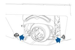
The hull drain plugs allow any water that may have collected in the hull of the amphibian to drain out. When the amphibian is on water, the hull should be sealed with the plugs provided. Always remove the plugs and allow to drain after use on water.
