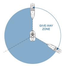
The illustration above indicates the "give-way" zone, relative to your amphibian, which is shown in the center of the diagram. You should give the right-of-way to all vessels to your starboard side in the "give-way" zone.
