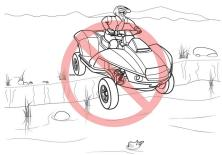
WARNING! Do not ride down a steep slope, off an undercut (for example, an eroded river bank,), a dock or other drop-off into the water. Ensure there are no obstacles or hazards at the entry point.
