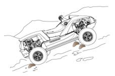
If it is necessary to park on a slope, block all four wheels to prevent rolling (for example, with chocks, rocks or logs) and, if possible, park the amphibian across the slope to prevent it from rolling.
