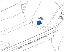
The amphibian has a mooring point located on each side.
