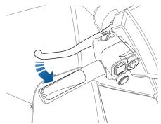
Apply the brake lever(s) smoothly with increasing pressure to slow or stop the amphibian.
