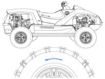
Your amphibian is fitted with directional tires. An arrow on the tire wall shows the direction of rotation. These tires must be fitted to rotate in the direction of the arrow when the vehicle is moving forward.
