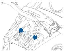
**11.** Remove screws (x2) securing the console center panel to the amphibian.
