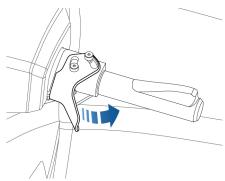
The throttle lever on the right handlebar controls the speed of the amphibian when it is being operated on both land and water.
