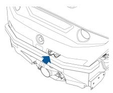
The bracket located at the rear of the amphibian is for mounting a flag only.
