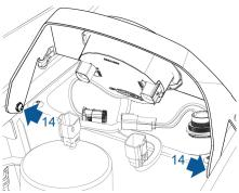
14. Remove screws (x2) securing the console center panel to the amphibian.
