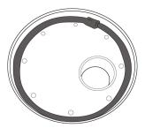
Apply a continuous bead of Deacon 3300 high temperature gasket compound to the inside of the muffler end cap. Start at a point between two stud holes and overlap the ends of compound by approximately 10mm.
