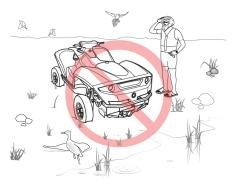
Avoid marshy areas and gravel surfaces. The amphibian can get stuck in marshy ground. If gravel surfaces are encountered, reduce speed to minimize the risk of debris entering the jet intake.
