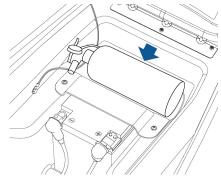
To ensure that your amphibian meets the requirements for operating on water, a fire extinguisher is located in the rear storage compartment.
