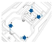
**3.** Remove the four screws securing the rear body panel to the amphibian.
