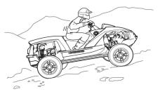
Before ascending a slope, slow down or stop to survey the terrain. When climbing a slope you must shift your weight toward the front wheels to help keep them on the ground. Move forward on the seat and lean forward.
