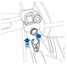
To reinstall the engine safety cut-off, insert the cut-off between the engine stop button and the handlebar.
