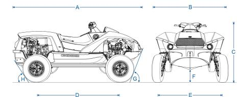
Overall length 3 244 mm 127.72 in А В Overall width 1 587 mm 62.5 in Overall height 1 359 mm 53.5 in С 70.5 in D Wheel base 1 790 mm Track width 55.5 in Е 1 410 mm Ground clearance 225 mm 8.9 in F 45° Approach angle G Departure angle Н 26°
