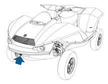
Only use the front eyelet for recovering the amphibian or securing to a trailer.
