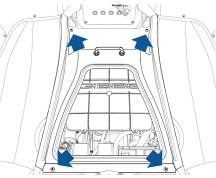
**9.** Remove the four screws securing the top of the upper body panel to the amphibian.
