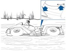
Approach the amphibian from either side and grab the handle below the seat.
