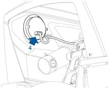
4. Disconnect the harness connector from each tail light and remove cable tie securing harness to body panel.
