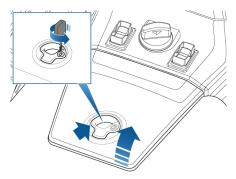
Lift the release ring and pull up to open the storage compartment.
