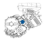
The identification number is located on the right side of the engine below the air intake box.
