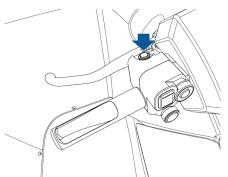
With the amphibian stationary and the throttle lever released, press and hold the reverse button to engage reverse. The instrument cluster will display an **R** to confirm that reverse is selected.
