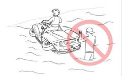
**NOTICE** The amphibian requires at least 3 ft (0.9 m) of water depth to deploy the wheels to their Land position. If the water is too shallow or a wheel strikes an underwater obstruction, the suspension will not deploy fully and an error will be displayed on the instrument cluster.
