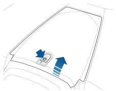
Push button, lift the latch and pull up to open the storage compartment.
