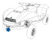
Secure the front of the amphibian using a ratcheting type tie-down strap attached to the front eyelet.
