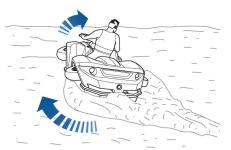
On-water, your amphibian is propelled and steered using a water jet. Turning the handlebars rotates the jet thrust nozzle, controlling the amphibian's direction. Steering control on water depends on the combination of handlebar rotation and thrust from the nozzle. Unlike a car, the amphibian requires some throttle to turn while in Marine mode.
