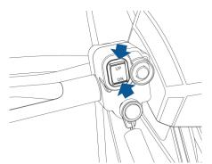
Use the gear selector switch to change gear.
