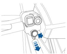
To stop the engine, press and hold the engine stop button or turn the ignition key to the Off position.
