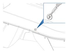
**3.** Located on the left side of the amphibian is a righting button. Position the righting loop of the lanyard over the righting button.
