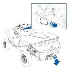
To move the amphibian in reverse on water, a lever is fitted to the amphibian that allows you to lower a reverse bucket across the water output. This reverse bucket is shaped to deflect the jet of high pressure water forward under the hull, which in turn pushes the amphibian in reverse.
