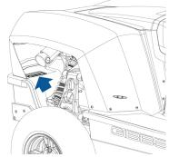
You can find the identification numbers stamped on a plate which is located on the hull in the right rear wheel well.
