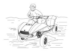
Terrain surface and speed are the major factors determining how the amphibian will react in a turn. Riding on loose, slippery or rough terrain (for example, snow, ice, mud, or gravel) makes it more likely for the amphibian to lose traction and skid or slide. This can result in a collision, or, if you unexpectedly regain traction, could result in the amphibian overturning. Stopping distances can also be longer.
