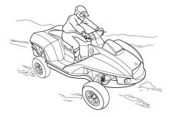
Do not descend a slope at high speed and avoid sudden braking or steering maneuvers as this could cause the amphibian to overturn.
