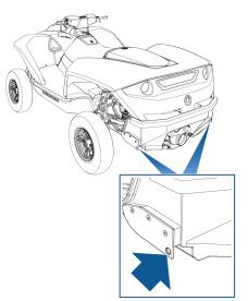
The rear of the amphibian should be secured using a ratcheting type tie-down strap attached to each rear sponson plate.
