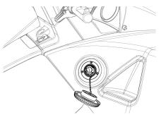
With the amphibian stationary and the engine off, slowly unscrew the fuel filler cap and allow the vapors to vent.
